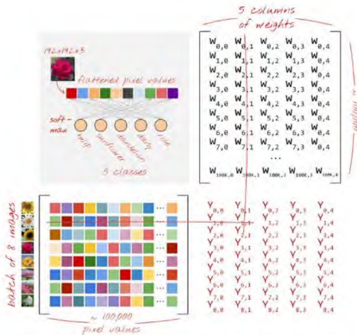
Illustration: a dense neural network layer as a matrix multiplication, with a batch of eight images processed through the neural network at once. Please run through one line x column multiplication to verify that it is indeed doing a weighted sum of all the pixels values of an image. Convolutional layers can be represented as matrix multiplications.
