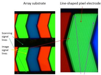
54. The products accused of infringing the '829 patent comprise a switching element for electrically connecting the pixel electrode and one of the image signal lines in response to a signal received from the scanning signal lines. For example, an examination of LGD's TFT-LCD included in Heesung LCM model no. HC49EQH-SLXA1-211X demonstrates this:
