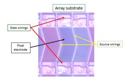
103. The products accused of infringing the '303 patent are configured such that the array substrate is provided with a switching element for switching a voltage applied to the pixel electrode from the source wiring based on a signal voltage fed from the gate wiring. For example, an examination of LGD's TFT-LCD included in Heesung LCM model no. HC49EQH-SLXA1-211X demonstrates this:
