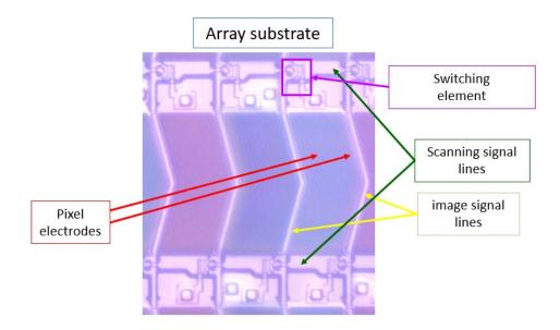
55. The products accused of infringing the '829 patent are configured such that of the pixel electrode and the common electrode, the electrode that is located adjacent to and parallel to one of the image signal lines or one of the scanning signal lines comprises an opaque conductor, and at least one of the other electrodes comprises a transparent conductor. For example, an examination of LGD's TFT-LCD included in Heesung LCM model no. HC49EQH-SLXA1-211X demonstrates this:
