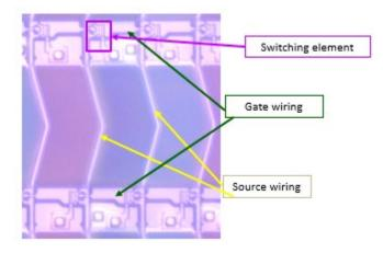
104. The products accused of infringing the '303 patent are configured such that the array substrate is provided with a common wiring formed between the two adjacent gate wirings. For example, an examination of LGD's TFT-LCD included in Heesung LCM model no. HC49EQH-SLXA1-211X demonstrates this:
