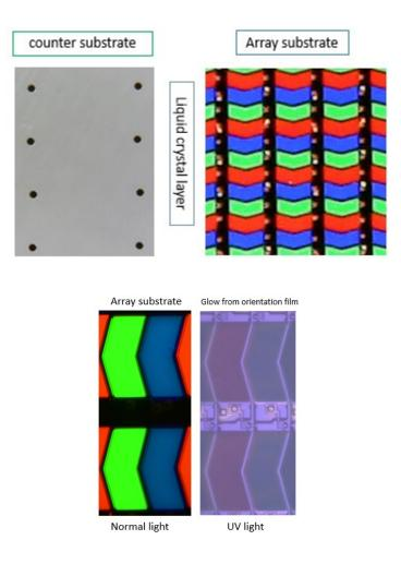
71. The products made using the method of manufacturing accused of infringing the '293 patent were made via a stripping step of stripping, by rubbing, a predetermined portion of the orientation film on the electrodes or lines once formed on the inner side of one or both of the substrates. The particular details are within Heesung and/or LGD's possession, custody, and control.
