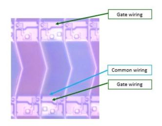
105. The products accused of infringing the '303 patent are configured such that the array substrate is provided with a common electrode being electrically connected to the common wiring and generating an electric field between the common electrode and the pixel electrode creating a voltage for driving the liquid crystal. For example, an examination of LGD's TFT-LCD included in Heesung LCM model no. HC49EQH-SLXA1-211X demonstrates this:
