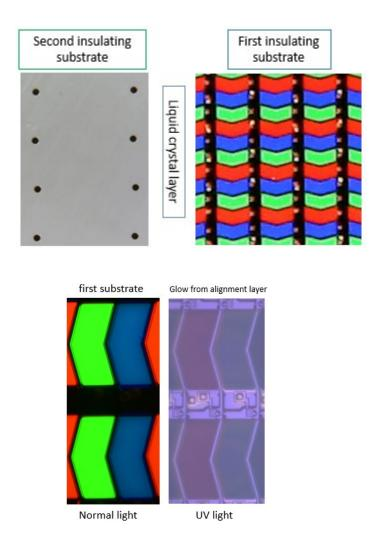
123. The products accused of infringing the '769 patent comprise alignment layers formed between the first insulating substrate and the liquid crystal layer and between the second insulating substrate and the liquid crystal layer, respectively, for aligning the liquid crystal layer. For example, an alignment layer, such as a polymer-based orientation film, between the second
