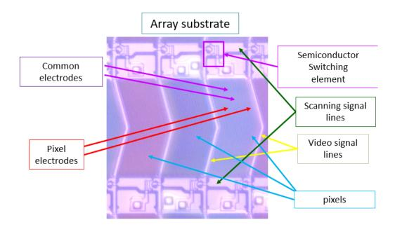
36. The products accused of infringing the '798 patent comprise a counter substrate arranged opposite the array substrate, and a liquid crystal layer sandwiched between the array substrate and the counter substrate. For example, an examination of LGD's TFT-LCD included in Heesung LCM model no. HC49EQH-SLXA1-211X demonstrates this:
