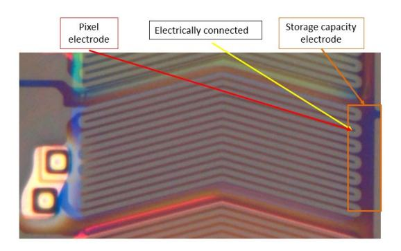
107. The products accused of infringing the '303 patent are configured such that the pixel electrode and the storage capacity electrode are layered so as to hold at least some part of the common wiring in between through an insulating layer. For example, an examination of LGD's TFT-LCD included in Heesung LCM model no. HC49EQH-SLXA1-211X demonstrates this:
