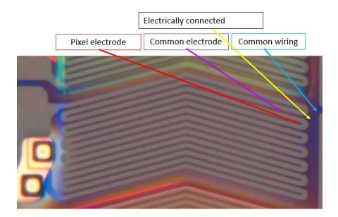
106. The products accused of infringing the '303 patent are configured such that the array substrate is provided with a storage capacity electrode electrically connected to the pixel electrode. For example, an examination of LGD's TFT-LCD included in Heesung LCM model no. HC49EQH-SLXA1-211X demonstrates this:
