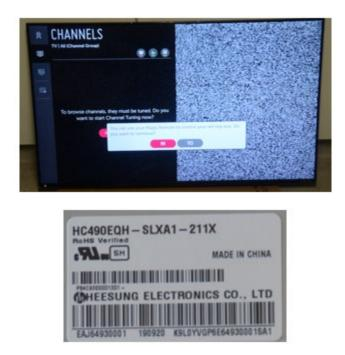
101. The products accused of infringing the '303 patent comprise an array substrate, an opposing substrate facing the array substrate, and liquid crystal held between the array substrate and the opposing substrate. For example, an examination of LGD's TFT-LCD included in Heesung LCM model no. HC49EQH-SLXA1-211X demonstrates this:
