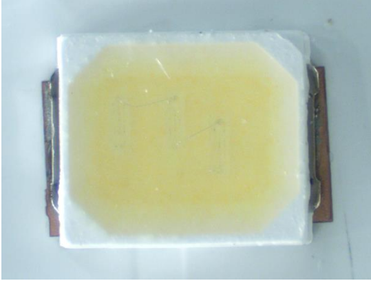
Figure 3A - 1 - LED Chip – Patriot Lighting Dusk-to-Dawn Outdoor Security Area Light
