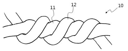
The aramid yarn would form loops during the twisting process, resulting in an unstable structure. When processing the raw HTC having this conventional
