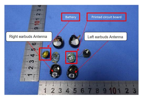
28. The Mod True Wireless earbuds also have at least one main printed circuit board, as indicated in the tear-down picture above, having circuitry for wireless radio communication, audio codec and earbud operation control. More specifically, on information and belief, the Mod True Wireless earbuds are "compatible with Bluetooth 5.2," "support[] the AAC and SBC
