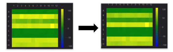
*Id.* The images above depict the impedance measured in each well of the 96-well CytoView-Z plate at a first time point (left) and a second time point (right), illustrating that the analysis is associated with individual wells of the plurality of wells.
