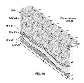
(shown in dashed lines in FIG. 1A) for receiving the different particulate mineral mixes via an open upwardly facing opening 132 of the mold 130." Exhibit 9, at 4:50-54.
