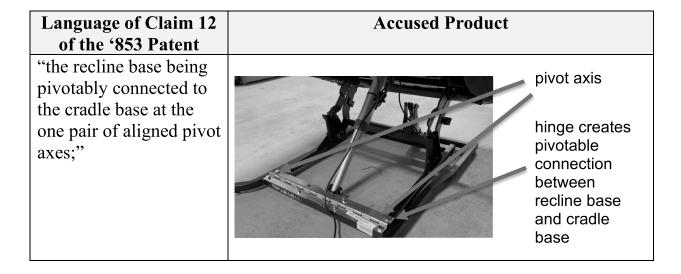
24. As shown in the comparison below of the claim language of the '853 Patent and images of the Accused Product, the Accused Product includes "a cradle actuator connected between the cradle base and the recline base for pivoting the recline base about the one pair of aligned pivot axes" as in claim 12 of the '853 Patent:
