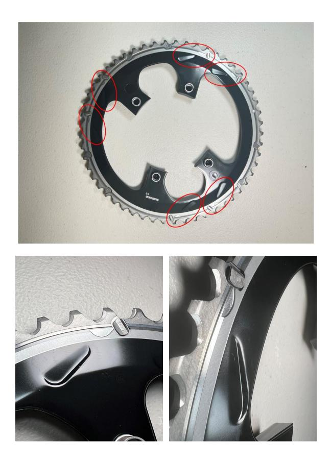
23. Each ramp has a ramp face on the inner surface of the chainring for receiving a link of an outside surface of a chain during an upshift.
