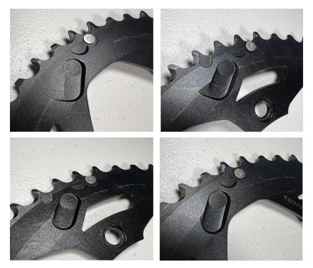
20. In normal operation, when upshifting from a smaller chainring, the derailleur moves the chain over to the inner surface of the larger rotating chainring, and the configuration of the ramps causes engagement of the ramp with at least one link of the bicycle chain at two or more distinct pivot points and lifts the chain toward the outer edge of the larger chainring, and the lifting is not assisted by (and precedes) engagement from any of the chainring teeth.
