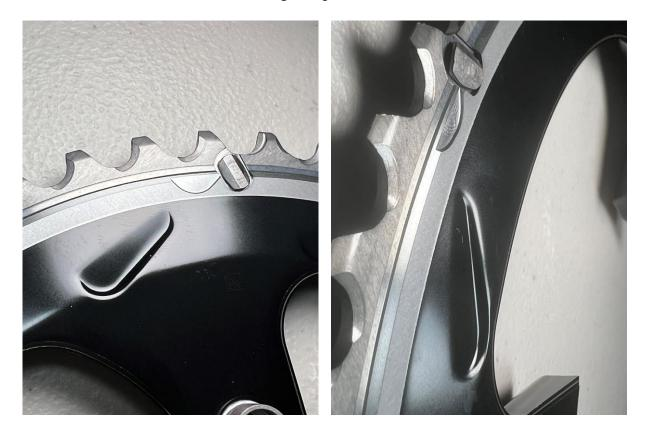
24. The REI Shimano accused chainrings have a first and second tooth of the plurality of teeth adjacent to the ramp face, the first tooth positioned before the second tooth relative to the direction of forward rotation of the bicycle chain ring, such that the ramp face is positioned a first distance from the first tooth and a second distance from the second tooth, and the first distance is greater than the second distance.
