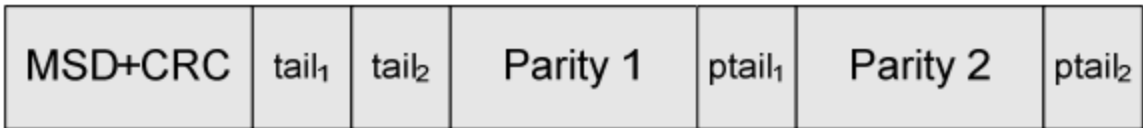
Figure 7: Channel coded bit buffer
