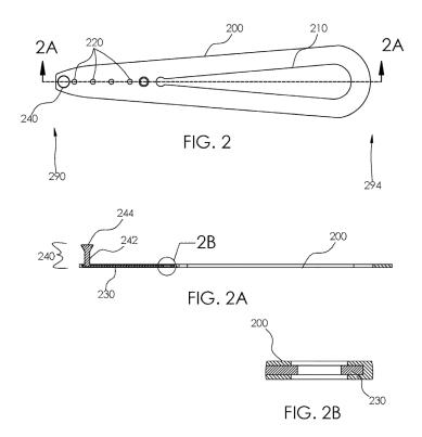
24. Regarding the rigid plate, the specification states that "[t]he rigid plate 230 may be a stiffener that may be embedded within the flexlatch 200" and "may establish the fixed opening width 294 by preventing a portion of the proximal 290 end of the flexlatch 200 from bending." The specification further states that "[i]n some embodiments, the rigid plate 230 may
