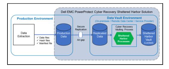
74. The Sheltered Harbor specifications require participants to protect critical data sets, including by creating dedicated, isolated environments which are physically separated from corporate networks and backup systems. Such data sets are converted for storage into Sheltered Harbor standardized format so that basic banking services can be quickly resumed for customers following an attack or failure. *See* Dell Sheltered Harbor Solution Brief.
