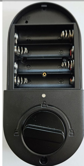
(photo of B0CGRRHXT6 smart lock (showing battery compartment holding 4 AA batteries)).
