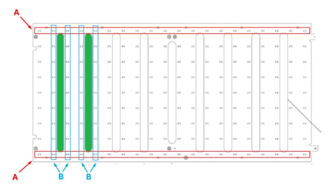
33. As shown in Exhibit C, the TILE Product includes a lighting sheet having a plurality of LEDs that emit light at a first color spectrum. For example, the LEDs can emit light having a color of 2200K, 2700K, 3000K, 3500K, 4000K, or 5700K.
