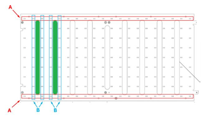
19. As shown in Exhibit C, the TILE Product includes a lighting sheet having a plurality of LEDs that emit light at a first color spectrum. For example, the LEDs can emit light having a color of 2200K, 2700K, 3000K, 3500K, 4000K, or 5700K.
