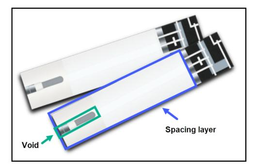
34. The void in the spacing layer at least partially defines a sample-receiving chamber
