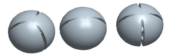
d. R3 Version (2020.11.26): Modified the mold shape of the water balloon body. Added sealing lips. The method of magnet fixation on PC plastic components was eliminated, and magnets were manually assembled onto the water balloon body.
