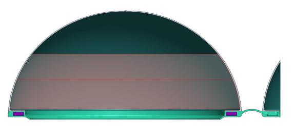
p. R15 Version (2022.4.20): To address issues such as magnet floating during mass production, the structure for fixing the magnets was modified.
