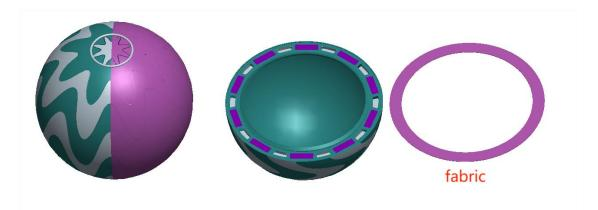
R11 Version (2021.6.23): Changed the outer diameter of the water balloon from 68mm to 58mm.
