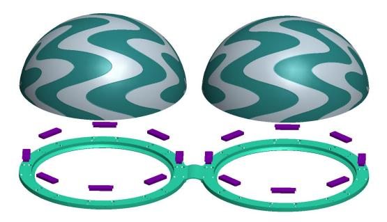
o. R14 Version (2021.11.20): After drop testing, it was found that the edges of the sphere were prone to breakage. Therefore, glue was added to the red area on the inner surface of the sphere.
