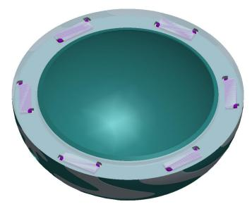
n. R13 Version (2021.9.27): Changed the water balloon structure. Split into First-color and Second-color segments connected by connecting straps to form a complete water balloon. The molding sequence is to embed the magnet into the First-color water balloon mold for molding. Then embed the formed First-color water balloon into the Second-color water balloon mold for molding.
