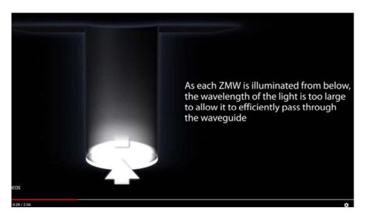
49. A Sequel loaded with a SMRT Cell 1M contains an excitation light source formed over the substrate.
