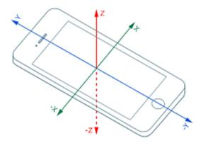
The iDriveAware application uses accelerometers with three or more axis sensors and/or gyroscopes with three or more axis sensors for monitoring three dimensional space(s) for representing the driver's movements (such as phone usage while driving, aggressive driving such
