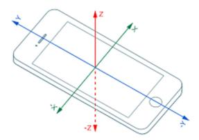
The telematics system includes code to monitor the x, y, and z axis of the accelerometers for measuring linear acceleration and gyroscopes for measuring angular velocity over time periods that are indicative of movement of the wireless communication device.
