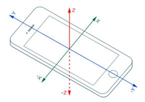
Defendant's telematics system uses wireless communication tracker devices equipped with accelerometers and/or gyroscopes with 3 or more axis sensors for monitoring three-dimensional space(s) for representing the vehicle's movements (such as fast acceleration, hard braking, cornering). The data from the 3-axis accelerometer and/or gyroscope data is measured by using time values for statistical analysis for determining human motions and activities.
