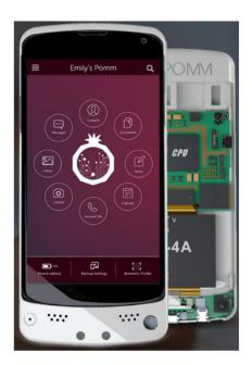
21. The POMM device possessed novel technology to mitigate user security risks through an isolated subsystem with its own processor, memory, and software/operating system. Isolated from the main functions of a smartphone, the POMM technology provided a physical, instead of a logical (*i.e.*, software based), segregation to protect sensitive user information, such as but not limited to, biometric data.
