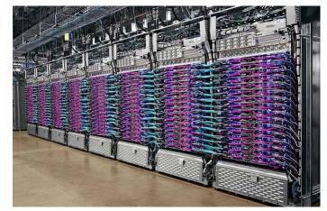
10. Plaintiff is informed and believes, and thereupon alleges, that Google achieves this improvement by bringing dialectric liquid to the four chips on each motherboard, each having a heat sink sitting atop each TPUv3 ASIC chip, allowing the coolant to circulate through the tubing and heat sinks to remove heat from the chips.
