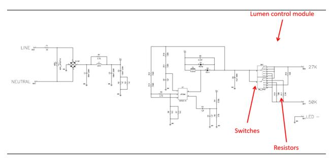
147. On information and belief, the Aviva Downlight comprises at least one light source coupled to the lumen control module, wherein the at least one light source emits a lumen output based on the current level received from the lumen control module. For example, as shown in Exhibit 25, the Aviva Downlight includes two LED arrays, labeled "27K" and "50K." Photographs of the two LED arrays are provided below:
