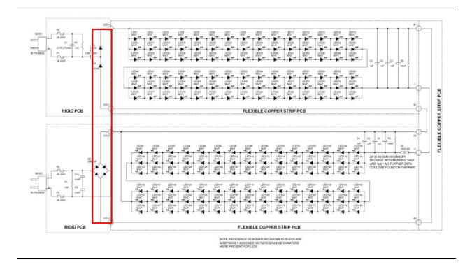
125. On information and belief, the SmartDrive LED Lamp comprises at least one light emitting diode coupled to outputs of the rectifier, wherein the first input of the rectifier is coupled to the first terminal via a capacitor. For example, the at least one light emitting diode, rectifier, first terminal, and capacitor of the SmartDrive LED Lamp are identified in Exhibit 23.
