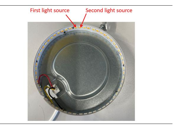
184. In addition, the first and second light sources have first and second color temperatures, as shown below:
