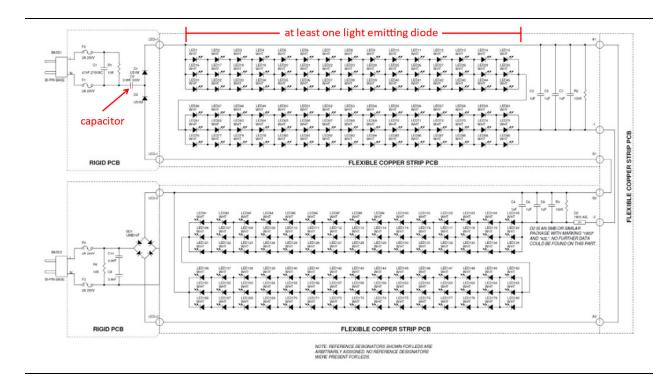
127. On information and belief, in the SmartDrive LED Lamp, the two first pins are interconnected via a first fuse, the capacitor being connected to one of the first pins, and the two second pins are interconnected via a second fuse. For example, the two first pins, first fuse, capacitor, two second pins, and second fuse of the SmartDrive LED Lamp are identified in Exhibit 23.
