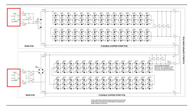
123. On information and belief, the SmartDrive LED Lamp comprises a rectifier with a first input coupled to the first terminal and with a second input coupled to the second terminal. For example, the rectifier of the SmartDrive LED Lamp is identified in Exhibit 23.
