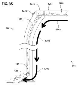
drains into an internal conduit provided in each corner post. After draining into this internal conduit, rainwater thereafter passes through an aperture provided in a lower portion of the respective corner post. One embodiment of this gutter system can be seen in the '187 Patent figure reproduced below:
