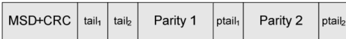
Figure 7: Channel coded bit buffer
