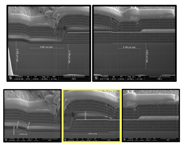
38. The composite images above show an n-type semiconductor layer having a surface, and a mesa located over a first portion of the surface of the n-type semiconductor layer,
