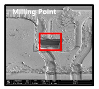
37. Below are cross-section images taken at the location of the red box in the image above, after the hole was milled (with annotations added for clarity).
