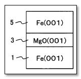
19. In some embodiments, the MgO layer is also formed with oxygen vacancy defects, such that the atomic ratio of Mg and O are no longer stoichiometric (that is, 1:1), but instead 1:x, where x < 1. The inventor recognized that when there are oxygen vacancy defects, a potential barrier height  $\Phi$  of the MgO tunnel barrier is reduced from 3.6 electron volts ("eV")
