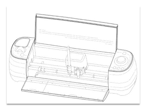
The broken lines immediately adjacent the shaded areas represent the bounds of the claimed design, while all other broken lines are directed to environment; the broken lines form no part of
