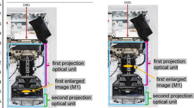
29. As shown above, the DMD of the GT3500HDR is located at one end of a collection of components that Maxell identifies as the GT3500HDR's first projection optical unit.
