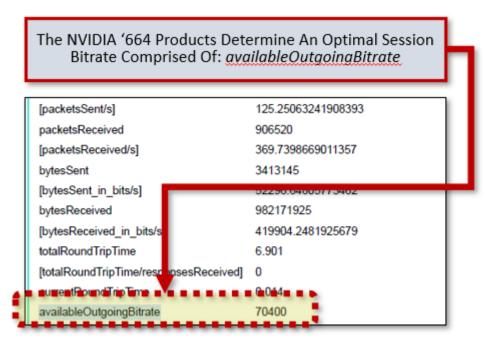
175. The NVIDIA '664 Products determine an optimal audio bitrate and an optimal video bitrate using the estimated network conditions. The NVIDIA '664 Products generate a target bitrate for audio and video data.
