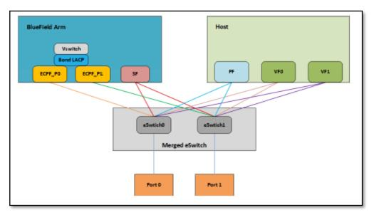
NVIDIA DOCA SWITCHING SUPPORT USER GUIDE, V2.2.0, NVIDIA DOCUMENTATION at 51 (October 2023) (showing how "Link Aggregation" switches between a first and second security link based on the health of the link).
