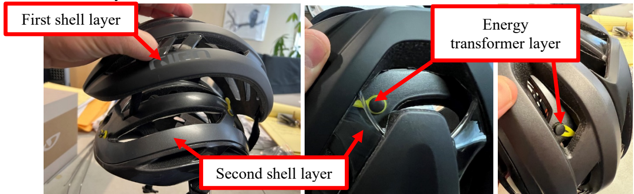
20 21 22 23 24 25 26 Fig. 34. Photos of Giro Aries Spherical helmet with first shell, second shell, and first 27 energy transformer layers labeled. Note the yellow elastic elements comprising the first energy transformer layer.
