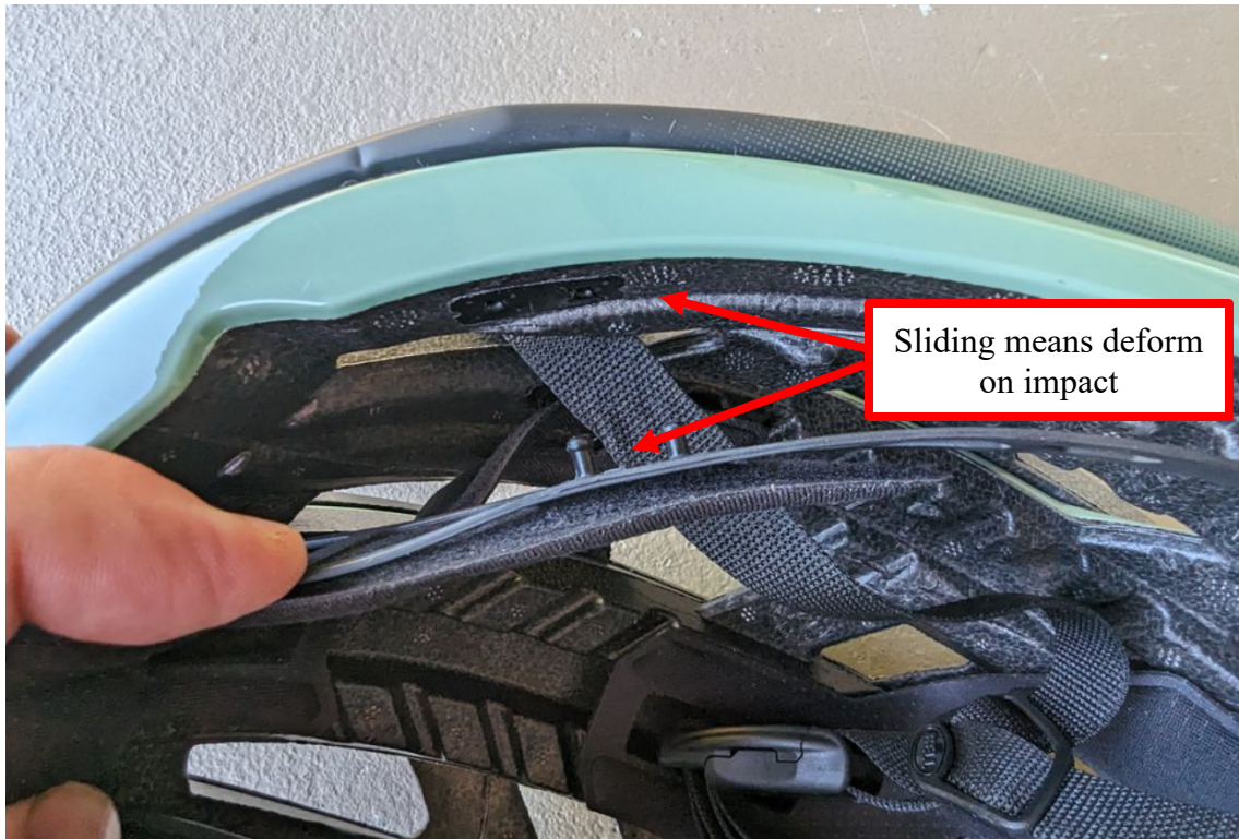
7 8 9 10 11 12 13 14 15 16 17 18 19 Fig. 20. Photo of the Bell XR Spherical inner and middle shells shown disconnected from 20 one another to illustrate the connection mechanism.
