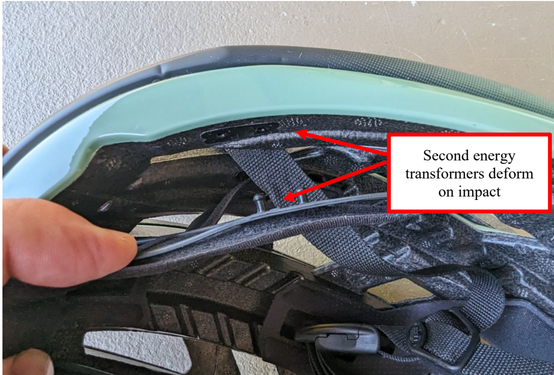
Fig. 75. Photo of the Bell XR Spherical second and third shells shown disconnected from one another to illustrate the connection mechanism (the second energy transformer).
