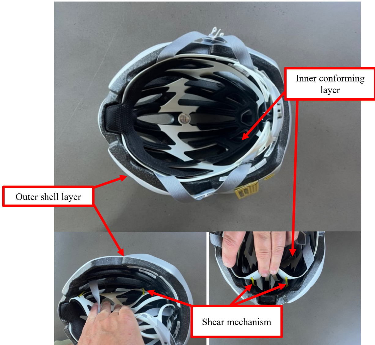
Fig. 79. Photos of the Bell Stratus MIPS helmet with outer shell, inner conforming layer, and shear mechanism labeled.
