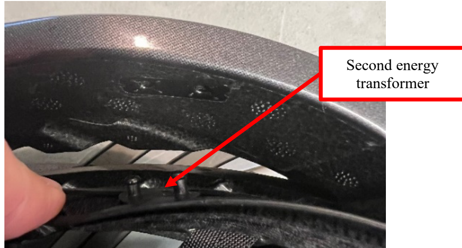
1 2 3 4 5 6 7 8 9 Fig. 73. Close-up photo of Giro Aries Spherical showing the disconnected second and third layers to illustrate the connection mechanism.
