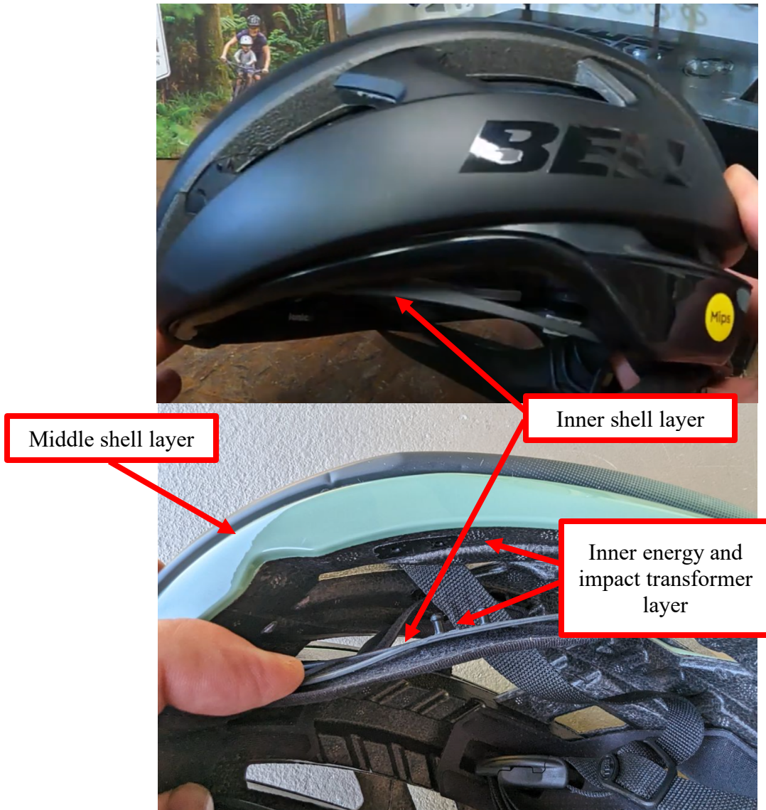
Fig. 15. Photos of the Bell XR Spherical helmet. The bottom photo depicts the inner shell layer disconnected from the middle shell layer to show the connection mechanism.
