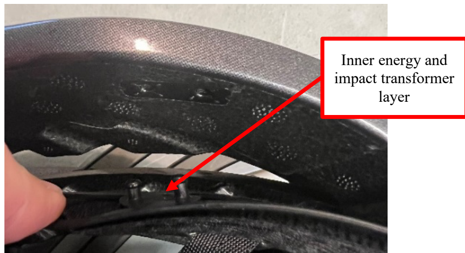
17 18 19 20 21 22 23 24 25 26 Fig. 18. Close-up photo of Giro Aries Spherical showing the disconnected inner shell and 27 middle shell layers to illustrate the connection mechanism.
