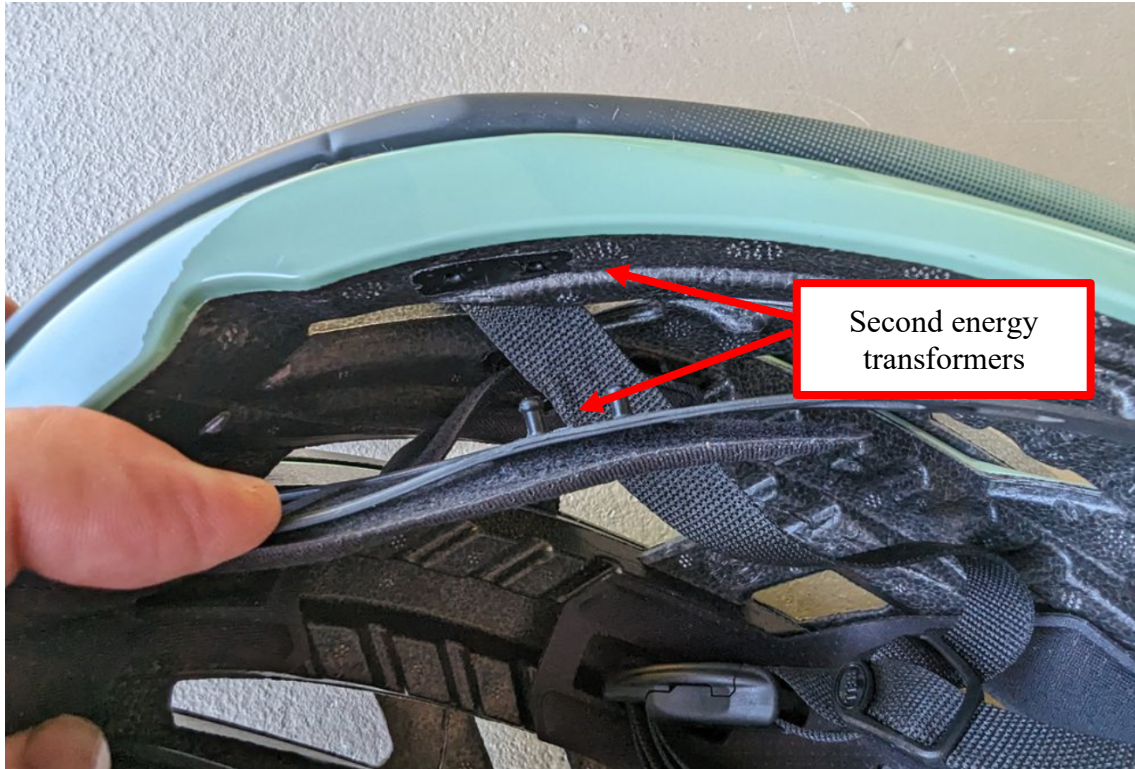
1 2 3 4 5 6 7 8 9 10 11 12 13 Fig. 72. Photo of the Bell XR Spherical helmet's second and third layers shown 14 disconnected from one another to illustrate the connection mechanism.
