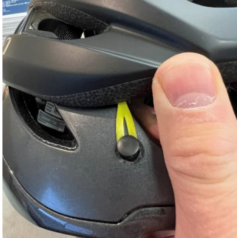
1 2 3 4 5 6 7 8 Fig. 48. Photos of the Giro Aries Spherical helmet. Note the yellow elastomeric energy 9 transformer.
