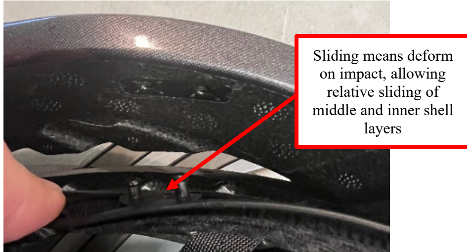
5 6 7 8 9 10 11 12 13 Fig. 21. Close-up photo of Giro Aries Spherical showing the disconnected inner shell and 14 middle shell layers to illustrate the connection mechanism.
