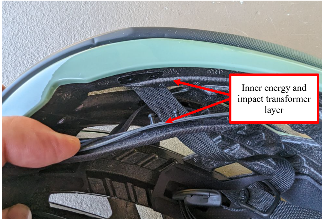
1 2 3 4 5 6 7 8 9 10 11 12 Fig. 17. Photo of the Bell XR Spherical helmet's inner and middle shells shown 13 disconnected from one another to illustrate the connection mechanism.
