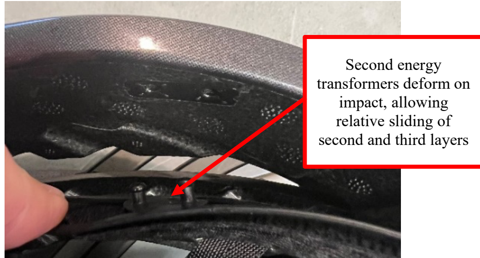
Fig. 76. Close-up photo of Giro Aries Spherical showing the disconnected second and third layers to illustrate the connection mechanism (the second energy transformer).
