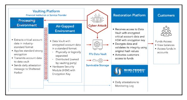
*see also* Reference Architecture (illustrating Sheltered Harbor compliant system and distributed architecture), as reproduced below:
