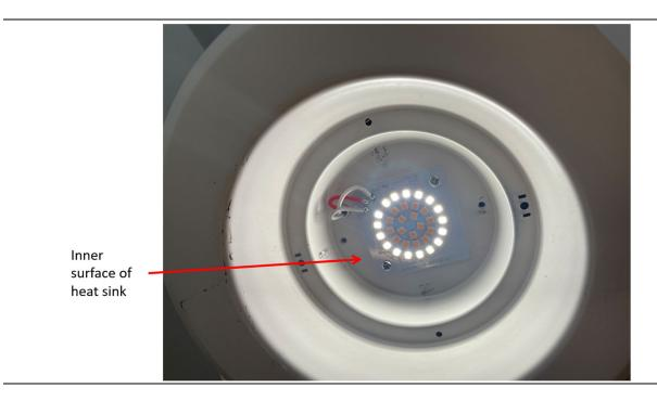
103. On information and belief, the Aviva Retrofit Downlight comprises at least one LED light source coupled to the inner surface of the heat sink, wherein the
