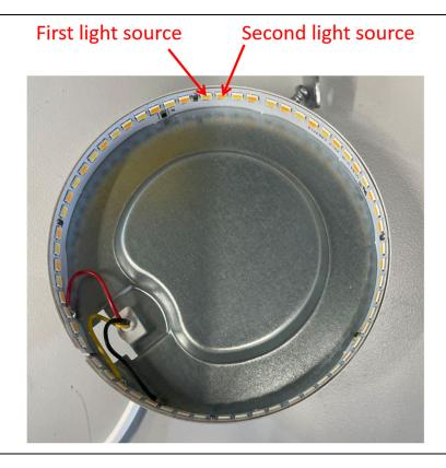
184. In addition, the first and second light sources have first and second color temperatures, as shown below:
