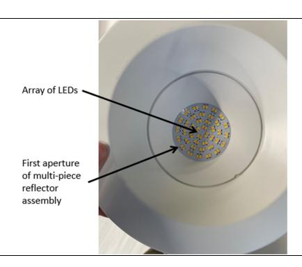
70. On information and belief the Advanta Downlight comprises a multipiece reflector assembly including a first reflector having said first aperture disposed in an upper portion of said first reflector and an opposed larger second aperture in a lower portion of said first reflector. For example, this limitation is shown below.
