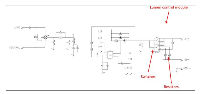
147. On information and belief, the Aviva Downlight comprises at least one light source coupled to the lumen control module, wherein the at least one light source emits a lumen output based on the current level received from the lumen control module. For example, as shown in Exhibit 25, the Aviva Downlight includes two LED arrays, labeled "27K" and "50K." Photographs of the two LED arrays are provided below:
