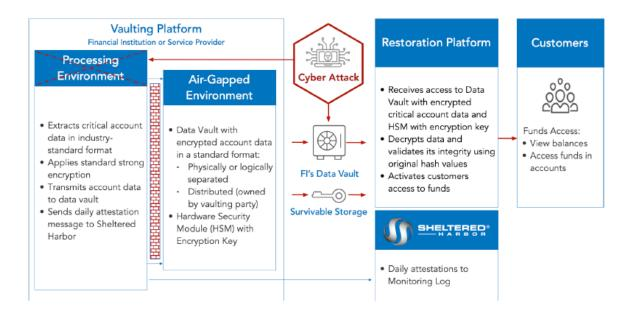
see also Reference Architecture (illustrating Sheltered Harbor compliant system and distributed architecture), as reproduced below:
